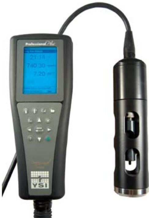
The Quatro is a new 4-port cable and bulkhead for the Professional Plus handheld instrument making it possible to measure conductivity and temperature, dissolved oxygen, and your choice of any two ISE's among pH, ORP, ammonium, nitrate or chloride.
