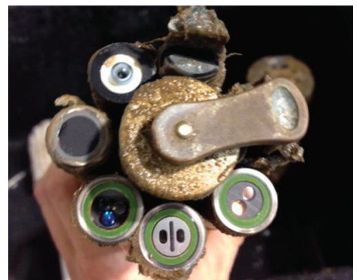
The YSI EXO multiparameter sondes minimize the effects of bio-fouling issues
