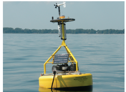
YSI buoy solution with EXO multiparameter sondes and WaterLOG Storm 3 datalogger
