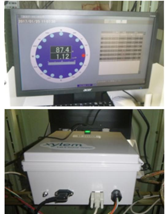
Fig 6: Real time data pertaining to current direction and speed acquired by Aqua Data Service is shown clearly on Desktop (TOP) linked to a data logger (BOTTOM).
