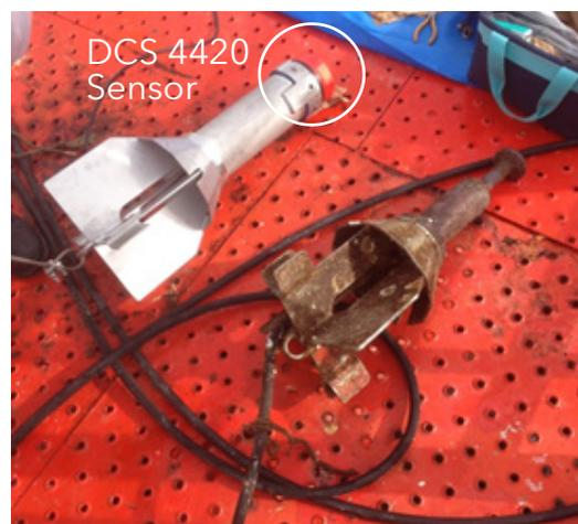
Fig3: Aanderaa DCS system from Xylem (LEFT) lying next to the previously installed EM sensor (RIGHT)
