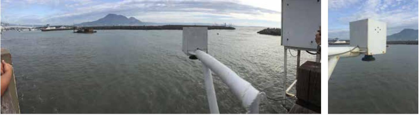
SINGAPORE: Singapore Cable Car uses a Nile Radar level sensor to monitor the height of the cable car cabins above mean sea level at Sentosa Singapore. The Singapore Cruise Centre is located nearby and has two berths of 310 metres and 270 metres handling international cruise ships with a height limit of 52 metres - thus continuous air gap monitoring is critical. The Storm3 Data Logger processes the data which is sent by radio to the control room.
