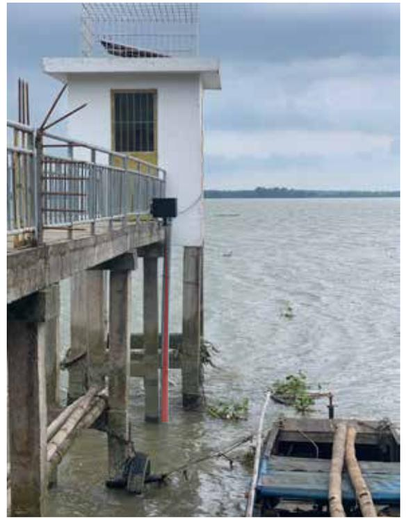
**Fig. 4.** MEKONG RIVER: Although the measurement footprint (highlighted in red) was subject to turbulent water and waves caused by vessels and wind, the Nile radar using the 181second measurement protocol is able to collect accurate and consistent data.
