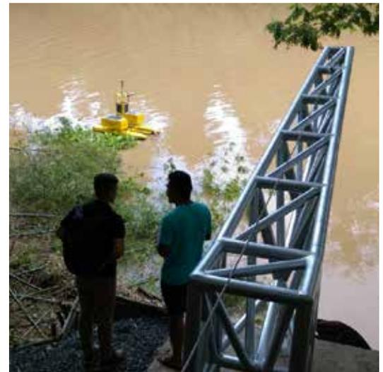
Figure 7: Custom support frame for high flow events
